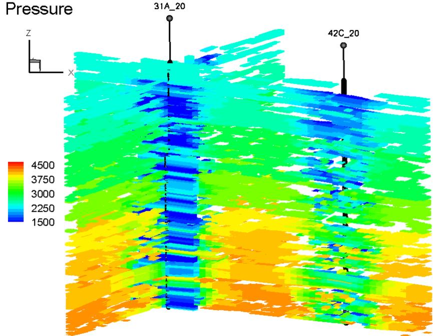
Cross-Section showing complex nature of pressure depletion
