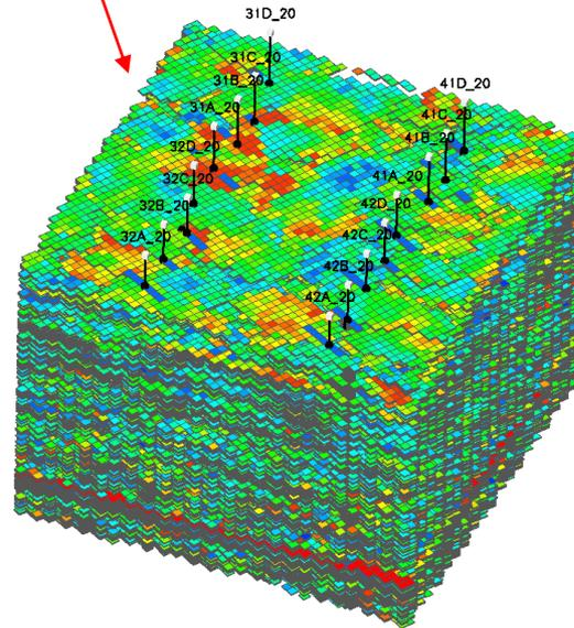
Simulated Hydraulic Fracture (Red = hydraulic fracture)
