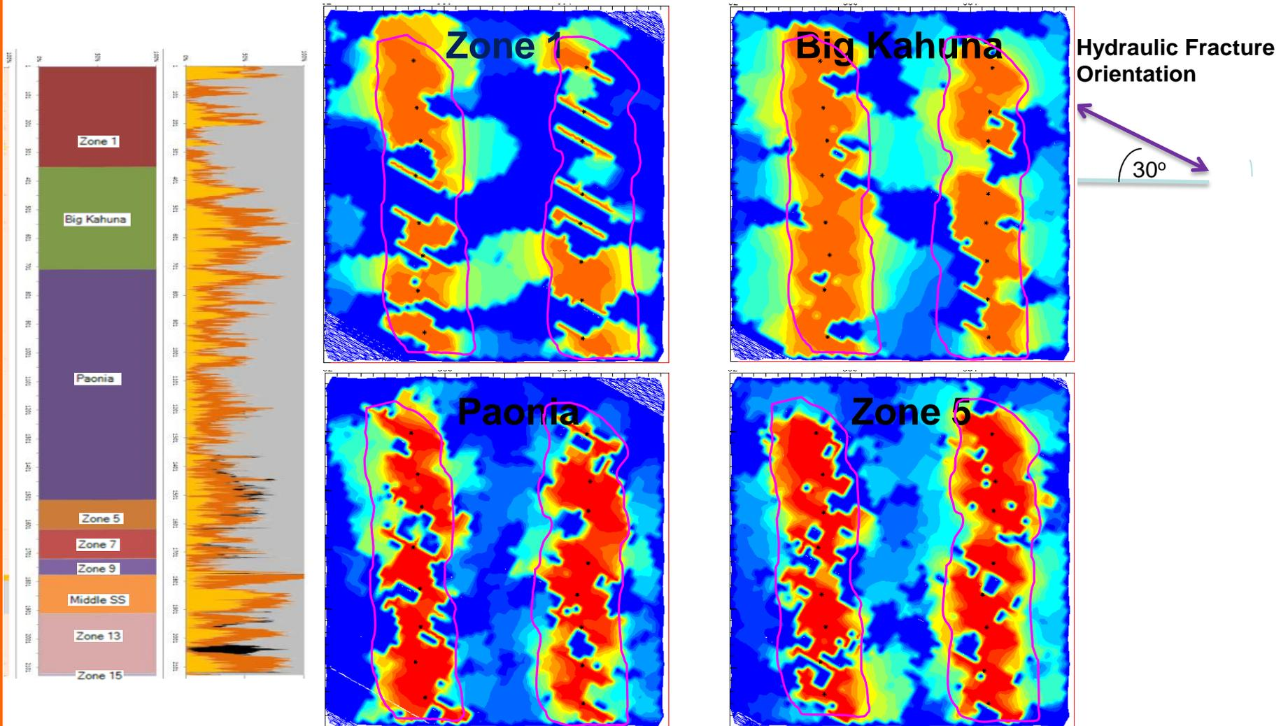
Recovery after 30 years, "optimal" hydraulic fractures, 25~30 ft thickness
