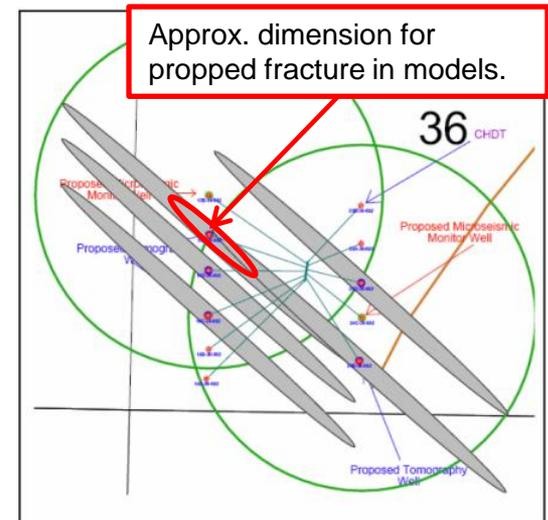
Figure 1. Gibson Gulch fracture mapping project setup.
